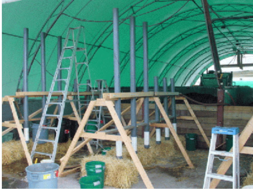
Figure 8 Test setup, showing racks to hold pipes, pipes of 2 lengths and slotted end sections
