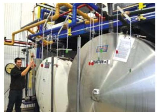
(above) Biodiesel is made in either of the two reactor tanks. The pipelines are colour-coded to clearly indicate what is in them.
